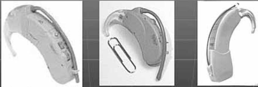
**Figure 2.** Examples of the first ear level FM receivers from early 1990's.
