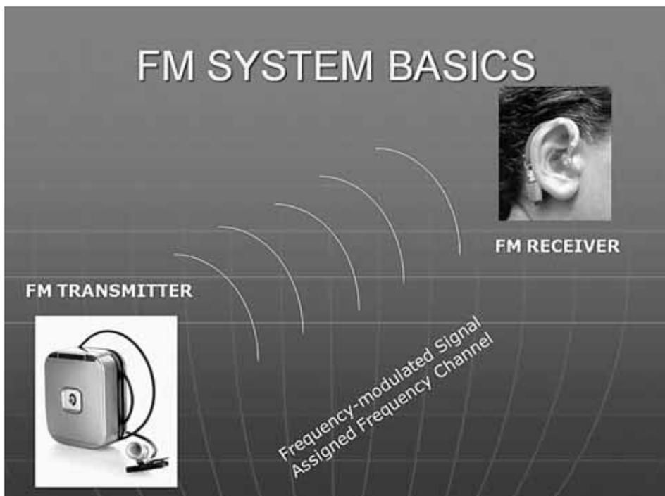
**Figure 1.** A basic FM system consists of a transmitter worn by the speaker and a receiver worn by the listener.
