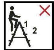
EN: Do not step off the side of the mobile platform ladder onto another surface.
