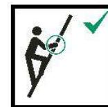
EN: Avoid work that imposes a sideways load on ladders, such as side-on drilling through solid materials.
