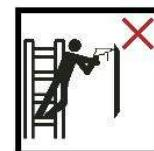
EN: Do not carry equipment which is heavy or difficult to handle while using a ladder.
