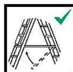
EN: Standing ladders shall not be used as a leaning ladder unless it is designed to do so.
