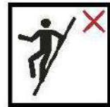
EN: Keep a secure grip on the ladder when ascending and descending.
