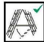
EN: Standing ladders shall not be used as a leaning ladder unless it is designed to do so.
