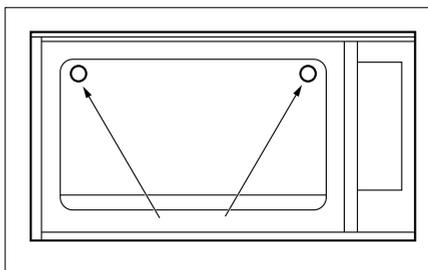
**IMPORTANT:** The oven's data plate is accessible even with the oven fully installed. The plate is visible simply by opening the door. Always quote the details from it to identify the appliance when ordering spare parts.
