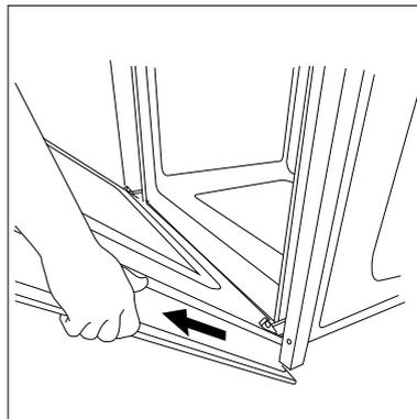
To replace fit the door, fit the hinges in their mountings and lower the two levers.
