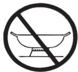
Do not place the pans directly on the burner.
