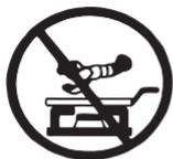
Do not use utensils that reflect a lot of heat downwards directly onto the grid.
