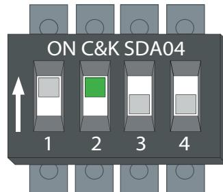
switch 2 → ON - Bluetooth communication enabled
