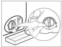
4. Turn the filter 180 degrees in anticlockwise direction to open it, without removing. Let the water flow out.
