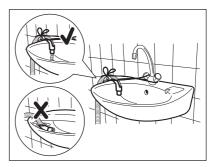
Make sure that the drain hose end is not immersed in the water. There may be a return of dirty water into the appliance.
