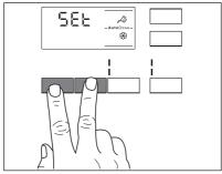
Touch related tank buttons to toggle function off and on. The display shows OFF when a tank is disabled or shows tank indicator when it is enabled.
