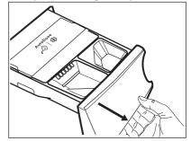
Put the powder detergent in the compartment W. When using liquid detergent, refer to "Manual filling the liquid detergent".
