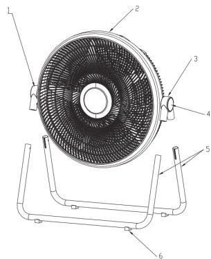
Insert the two ends of the U-shaped tubes into the left and right brackets respectively.
