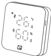
Smart controller with T&H sensor
